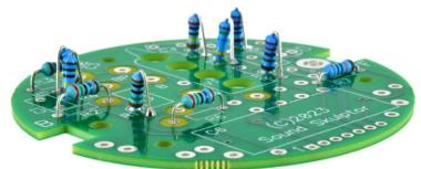
Control the resistor values with a digital multimeter, except R2, R3, R6 which are too high for most DMM's.. Bend the leads at 0.4" with a lead forming tool.
