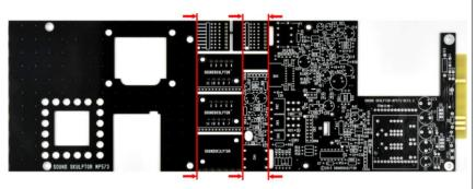
There are two additional safety PCB's available: One input transformer PCB and one output transformer connector PCB. These won't be used for this build.
