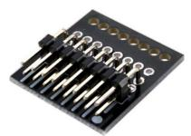
Place the 2x8 pins, 90° connector on the output transformer PCB, on the side where it is drawn. Solder.
