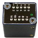
Remove the 2 screws from the transformer pin side and place 2 nylon washers over the holes
