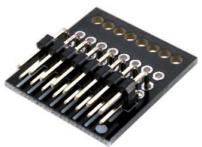
Place the 2x8 pins, 90° connector on the output transformer PCB, on the side where it is drawn. Solder.
