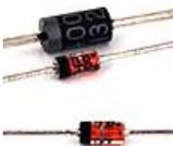
Add D1, D4 to D7. Use a lead forming tool to bend the leads at 0.4”.
