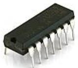
Insert U1, U2, U3 and U4 and solder. You will need to bend the pins slightly inwards before inserting.
