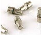
Solder the 7 pin sockets for the DOA. Solder one at a time. Insert one socket, turn over the PCB and press against a solid but flexible surface like cork or dense foam then solder. The correct positioning of the sockets is very important for easy insertion of the DOA.
